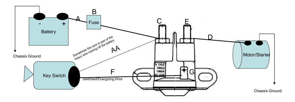
Note: Do not remove nut from stud (C) or stud (E). Do not bend spade (G)
