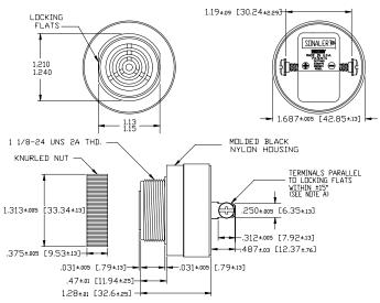
NOTE A: TERMINALS-032 BRASS TIN PLATED, TAPPED FOR #6-32 SCREW. TWO #6-32 NICKEL PLATED BRASS SCREWS INCLUBED. WILL ACCEPT 1/4' QUICK CONNECT. NOTE B: MOUNTING- REMOVE BLACK PLASTIC NUT AND INSERT THREADED FRONT THROUGH 1.25' HOLE PUNCHED IN PANEL, IF DRIENTATION IS NEEDED, NOTE LOCKING FLATS ON DRAVING. SCREW NUT BACK ON. DO NOT OVERTIGHTEN.
