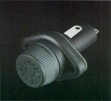
Equipped with "O"-ring seals for applications requiring waterproof protection. Holders mount in panels up to ½" (6.4mm) thick. Military version designated FHN23W. U.L. Recognized (File No. E14853, Guide No. IZLT2).
