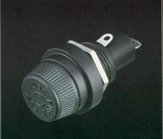
For supplementary protection of transformers, relays, ballasts, and small motors. Screw type knob. HPL-B has solder type terminals; HPM ½" quick-connect. HPM is U.L. Recognized and CSA Listed (U.L. File No. E14853, Guide No. IZLT2; CSA File No. 47235, Class 6225-01).
