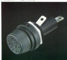
For supplementary protection of transformers, relays, ballasts, and small motors. Mount in ½" (12.7mm) knock-outs with locknut. Bayonet type knob. Combination ¼" (6.4mm) quick-connect/solder terminals. U.L. Recognized File No. E14853, Guide No. IZLT2.
